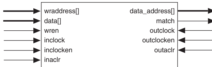
Figure 23. APEX 20KC CAM Block Diagram
