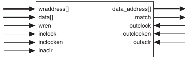
Figure 23. APEX 20KC CAM Block Diagram
