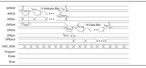
Figure 5-4. UFM Program Waveforms
