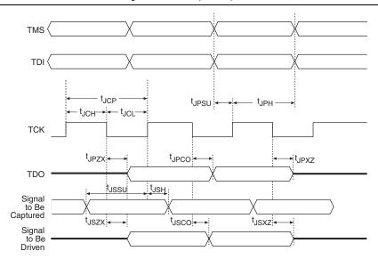
Figure 13–6. IEEE Std. 1149.1 Timing Waveforms (Note 1)
