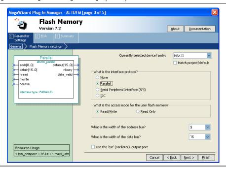
The UFM block's internal oscillator is always running when the altufm\_parallel magafunction is instantiated for read/write interface. The UFM block's internal oscillator is disabled when the altufm\_parallel megafunction is instantiated for read only interface.
