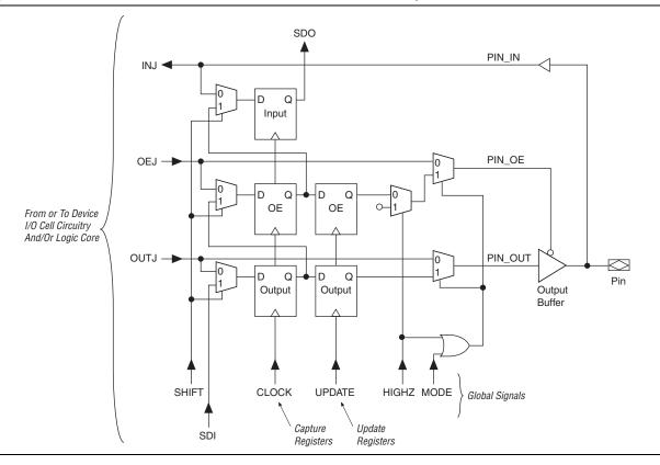
Table 13–2 describes the capture and update register capabilities of all boundary-scan cells within MAX II devices.
