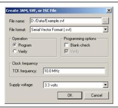
Before creating the SVF File, you must open the Programmer in the Quartus II and add the Programmer Object File (.pof) for all the devices in the chain into the programmer. Each POF corresponds to a targeted device, respectively.
