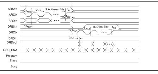
Figure 9–8. UFM Stream Read Waveforms
