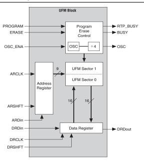
Table 9–4 summarizes the MAX II UFM block input and output interface signals.
