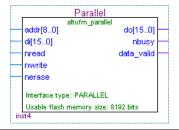
Figure 9–42 shows page 3 of the altufm MegaWizard Plug-In Manager, selecting the Parallel Interface as the interface. On this page, you can choose whether to implement the Read/Write mode or Read Only mode for the UFM. You also have an option to choose the width for address bus (up to 9 bits) and for the data bus (up to 16 bits). You can specify the initial content of the UFM block on page 4 of the altufm MegaWizard Plug-In Manager as discussed in "Creating Memory Content File" on page 9–40.
