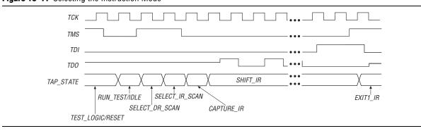
The TDO pin is tri-stated in all states except the SHIFT\_IR and SHIFT\_DR states. The TDO pin is activated at the first falling edge of TCK after entering either of the shift states and is tri-stated at the first falling edge of TCK after leaving either of the shift states.
