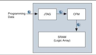
In real-time ISP mode, the user flash memory (UFM), programmable logic, and I/O pins remain operational while programming of the CFM is in progress. The contents of the CFM will not download into the SRAM after the successful programming of the CFM. Instead, the device waits for a power cycle to occur. The normal power-up sequence occurs (CFM downloads to SRAM at power-up) and the device enters user mode after  $t_{\rm CONFIG}$  time. Figure 12–2 shows the flow of real-time ISP.
