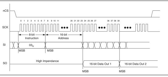
Figure 9–27 shows the READ operation sequence for Base mode.
