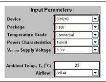
Table 17–1 describes the values that must be specified in the Input Parameter section of the PowerPlay Early Power Estimator spreadsheet.
