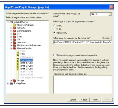
The altufm MegaWizard Plug-In Manager has separate pages that apply to the MAX II UFM block. During compilation, the Quartus II Compiler verifies the altufm parameters selected against the available logic array interface options, and any specific assignments.
