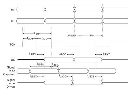
Table 5–31 shows the JTAG Timing parameters and values for MAX II devices.
