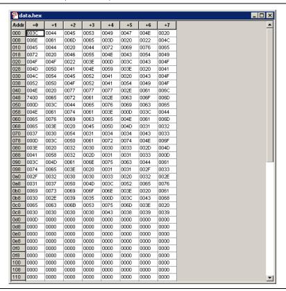
This memory content file is then included using the altufm megafunction. On the Tools menu, click **MegaWizard Plug-In Manager**. The memory content file (**data.hex**) is included on page 5 of the altufm megafunction (Figure 9–48). Click **Yes**, and use this file for the memory content file. Click **Browse** to include the memory content file.
