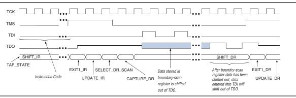
Figure 13–9. SAMPLE/PRELOAD Shift Data Register Waveforms
