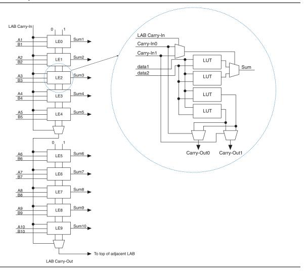
The Quartus II software automatically creates carry chain logic during design processing, or you can create it manually during design entry. Parameterized functions such as LPM functions automatically take advantage of carry chains for the appropriate functions. The Quartus II software creates carry chains longer than 10 LEs by linking adjacent LABs within the same row together automatically. A carry chain can extend horizontally up to one full LAB row, but does not extend between LAB rows.
