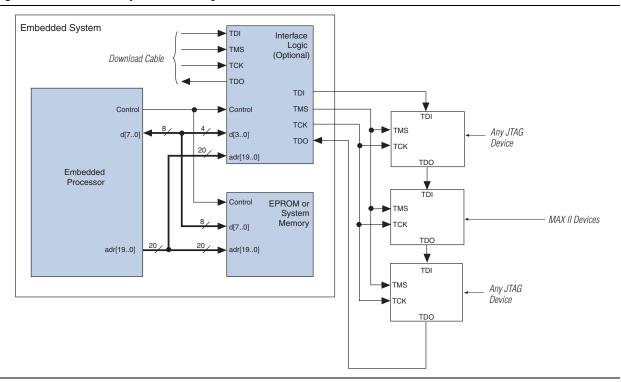
Figure 14–1. Embedded System Block Diagram
