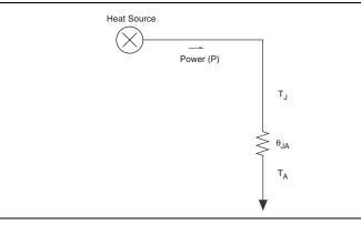
The PowerPlay Early Power Estimator spreadsheet determines the junction-to-ambient thermal resistance ( $\theta_{JA}$ ) based on the device, package, and airflow selected in the main input parameters.
