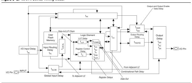
The timing characteristics of any signal path can be derived from the timing model and parameters of a particular device. External timing parameters, which represent pin-to-pin timing delays, can be calculated as the sum of internal parameters.
