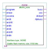
Figure 9–44 shows page 3 of the altufm MegaWizard Plug-In Manager, selecting **none** for the interface protocol. By selecting **none**, all the other options are grayed out or unavailable to you. However, you still can specify the initial content of the UFM block on page 4 of the altufm MegaWizard Plug-In Manager as discussed in "Creating Memory Content File" on page 9–40.
