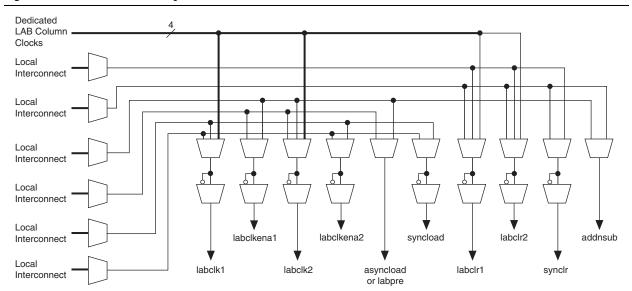
Figure 2–5. LAB-Wide Control Signals
