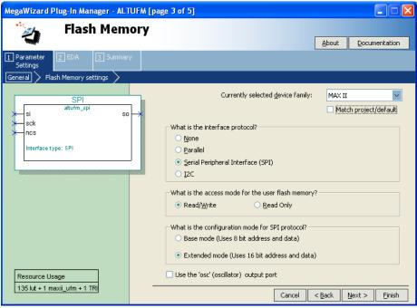
The UFM block's internal oscillator is always running when the altufm\_spi megafunction is instantiated for read/write interface. The UFM block's internal oscillator is disabled when the altufm\_spi megafunction is instantiated for read only interface.
