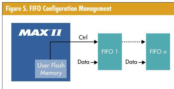
Figure 5. FIFO Configuration Management
