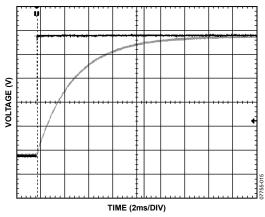
Figure 16. Turn-On Time:  $C_X$ ,  $C_Y = 0.1 \mu F$ , Time Scale = 2 ms/div
