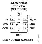
Figure 4. ADW22035 Pin Configuration
