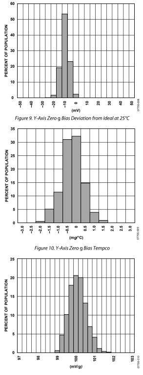
Figure 11. Y-Axis Sensitivity at 25°C
