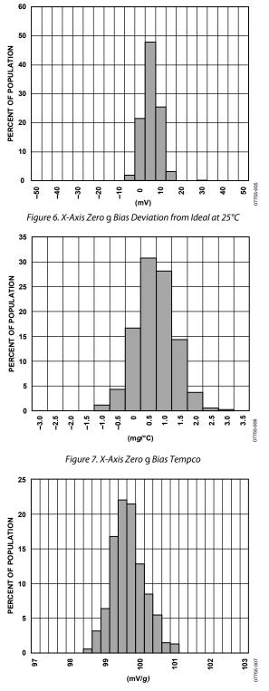
Figure 8. X-Axis Sensitivity at 25°C
