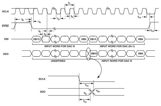
Figure 23. Daisy-Chaining Timing Diagram
