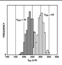
TPC 10.  $I_{DD}$  Histogram with  $V_{DD} = 3 V$  and  $V_{DD} = 5 V$
