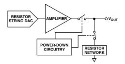
Figure 10. Output Stage During Power-Down
