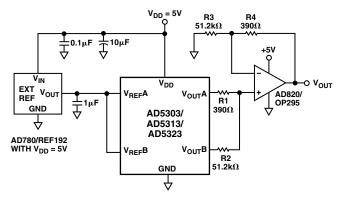
Figure 21. Coarse/Fine Adjustment
