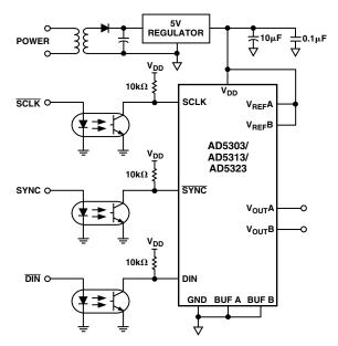
Figure 18. AD5303/AD5313/AD5323 in an Opto-Isolated Interface
