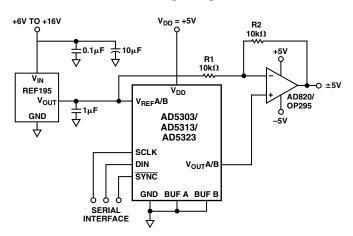
Figure 17. Bipolar Operation Using the AD5303/ AD5313/AD5323
