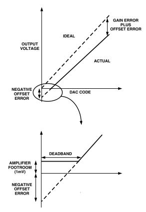
Figure 3. Transfer Function with Negative Offset
