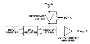
Figure 5. Single DAC Channel Architecture
