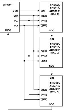
\*ADDITIONAL PINS OMITTED FOR CLARITY Figure 22. Daisy-Chain Mode
