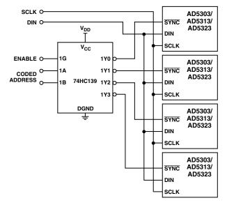
Figure 19. Decoding Multiple AD5303/AD5313/ AD5323 Devices in a System
