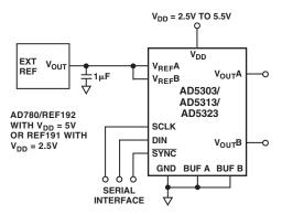
Figure 15. AD5303/AD5313/AD5323 Using External Reference
