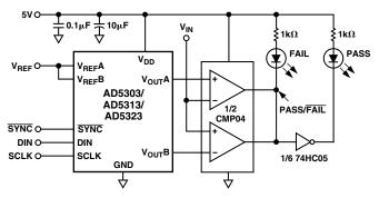
Figure 20. Window Detector Using AD5303/ AD5313/AD5323
