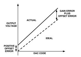
Figure 4. Transfer Function with Positive Offset
