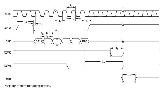
Figure 2. Serial Interface Timing Diagram
