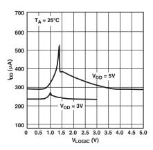
*TPC 15. Supply Current vs. Logic Input Voltage*
