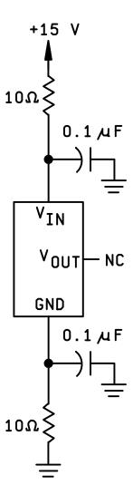
FIGURE 2. Radiation exposure circuit.
