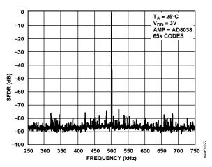
Figure 28. Narrow-Band Spectral Response,  $f_{OUT} = 500 \text{ kHz}$ , Clock = 25 MHz
