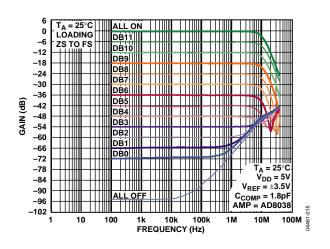
Figure 16. Reference Multiplying Bandwidth vs. Frequency and Code
