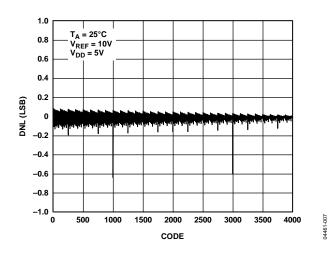
Figure 8. Differential Nonlinearity (DNL) vs. Code (12-Bit DAC)
