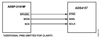
Figure 41. ADSP-2191M SPI to AD5415 Interface
