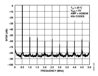
Figure 26. Wideband SFDR,  $f_{OUT} = 500 \text{ kHz}$ , Clock = 10 MHz
