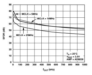
Figure 24. Wideband SFDR vs. four Frequency
