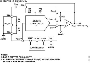
Figure 34. Unipolar Operation
