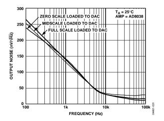
Figure 32. Output Noise Spectral Density
