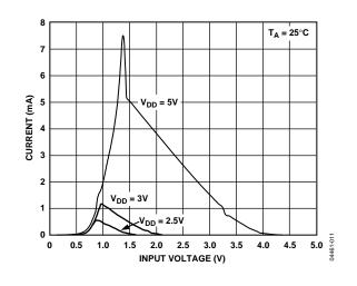
Figure 12. Supply Current vs. Logic Input Voltage
