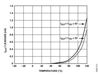
Figure 13. Iout1 Leakage Current vs. Temperature
