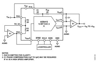
Figure 35. Bipolar Operation
