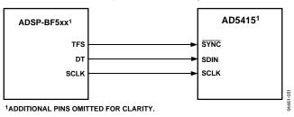
Figure 44. ADSP-BF504 to ADSP-BF592 Device Family SPORT to AD5415 Interface (ADSP-BFxx Denotes the ADSP-BF504 to ADSP-BF592)
