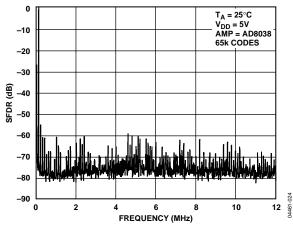
Figure 25. Wideband SFDR,  $f_{OUT} = 100 \text{ kHz}$ , Clock = 25 MHz
