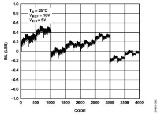
Figure 7. Integral Nonlinearity (INL) vs. Code (12-Bit DAC)
