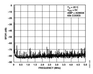
Figure 27. Wideband SFDR,  $f_{OUT} = 50$  kHz, Clock = 10 MHz
