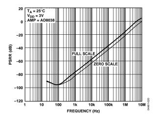
Figure 21. Power Supply Rejection Ratio vs. Frequency
