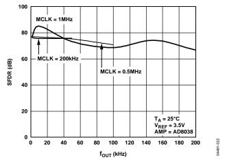
Figure 23. Wideband Spurious-Free Dynamic Range (SFDR) vs. four Frequency
