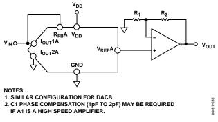
Figure 36. Single-Supply Voltage Switching Mode
