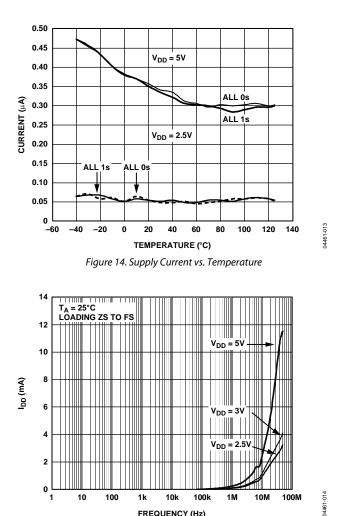
FREQUENCY (Hz) Figure 15. Supply Current vs. Update Rate
