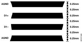
Figure 61. Arrangement of Signal Tracks
