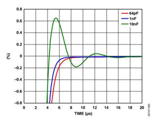
Figure 24. Zoomed in Settling for a ¼ to ¾ Output Voltage Step
