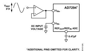
Figure 41. Pseudo Differential Mode Connection Diagram
