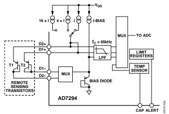
Figure 45. Internal and Remote Temperature Sensors
