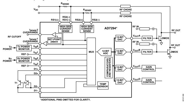
Figure 59. Typical HPA Monitor and Control Application
