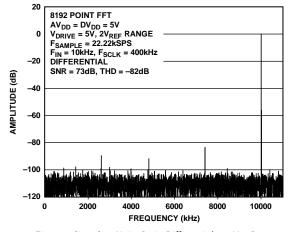
Figure 9. Signal-to-Noise Ratio Differential,  $2 \times V_{REF}$  Range
