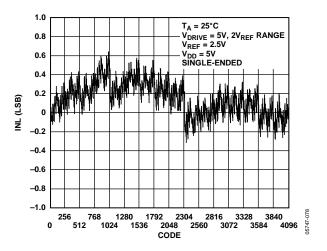
Figure 12. ADC INL Single-Ended,  $2 \times V_{REF}$  Range
