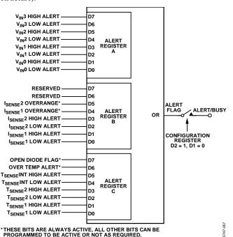
Figure 57. Alert Register Structure
