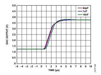
Figure 23. Settling Time for a ¼ to ¾ Output Voltage Step
