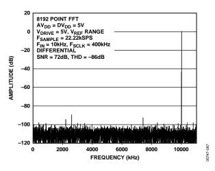
Figure 8. Signal-to-Noise Ratio Differential, VREF Range
