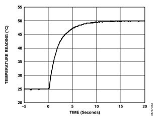
Figure 28. Response of the AD7294 to Thermal Shock Using 2N3906 (2N3906 Placed in a Stirred Oil Bath)
