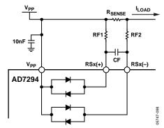
Figure 43. Current Sense Filtering (RS<sub>X</sub> Can Be Either RS1 or RS2)
