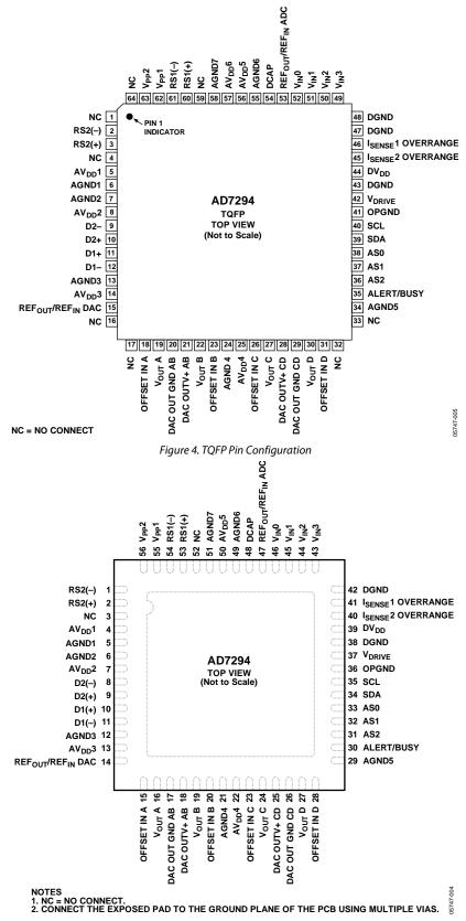
Figure 5. LFCSP Pin Configuration
