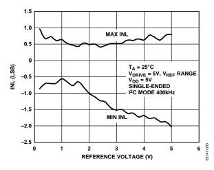
Figure 18. ADC INL vs. Reference Voltage
