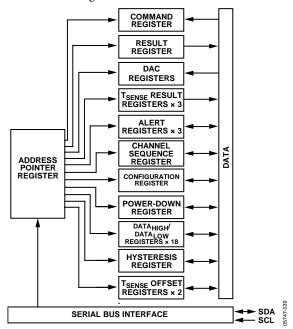
Figure 49. AD7294 Register Structure
