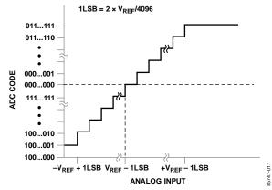
Figure 36. Differential Transfer Characteristic with V<sub>REF</sub> ± V<sub>REF</sub> Input Range
