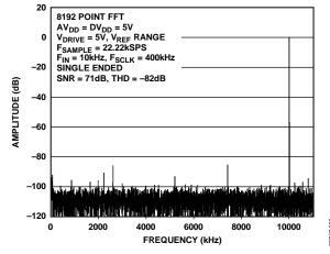
Figure 6. Signal-to-Noise Ratio Single-Ended, VREF Range
