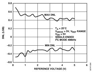
Figure 19. ADC DNL vs. Reference Voltage
