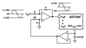
Figure 37. Single-Ended Mode Connection Diagram
