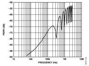
Figure 33. I<sub>SENSE</sub> Power Supply Rejection Ratio vs. Supply Ripple Frequency Without V<sub>PP</sub> Supply Decoupling Capacitors for a 500 mV Ripple
