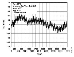
Figure 15. ADC INL Differential, VREF Range
