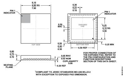
Figure 63. 56-Lead Lead Frame Chip Scale Package [LFCSP] 8 mm × 8 mm body and 0.75mm Package Height (CP-56-11) Dimensions shown in millimeters
