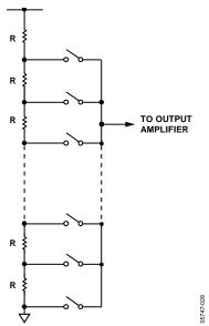
Figure 48. Resistor String Structure
