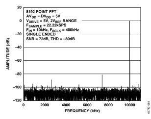
Figure 7. Signal-to-Noise Ratio Single-Ended,  $2 \times V_{REF}$  Range
