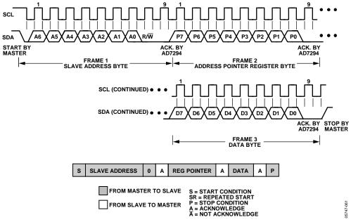
Figure 51. Single Byte Write Sequence
