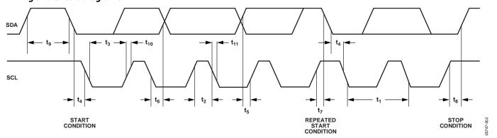
Figure 2. I<sup>2</sup>C-Compatible Serial Interface Timing Diagram
