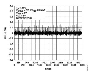
Figure 17. ADC DNL Differential,  $2 \times V_{REF}$  Range
