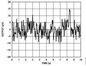
Figure 22. 0.1 Hz to 10 Hz DAC Output Noise (Code 800)
