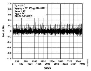
Figure 13. ADC DNL Single-Ended,  $2 \times V_{REF}$  Range
