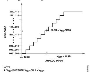
Figure 35. Single-Ended Transfer Characteristic
