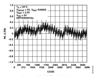
Figure 14. ADC INL Differential,  $V_{\it REF}$  Range
