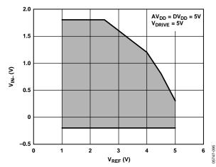
Figure 40. V<sub>IN-</sub> Input Range vs. V<sub>REF</sub> in Pseudo Differential Mode
