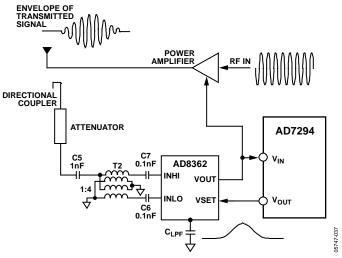
Figure 60. Setpoint Controller Operation
