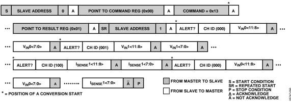
Figure 56. Command Mode Operation
