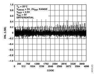
Figure 16. ADC DNL Differential,  $2 \times V_{REF}$  Range
