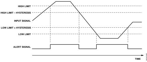
Figure 58. Limit Checking
