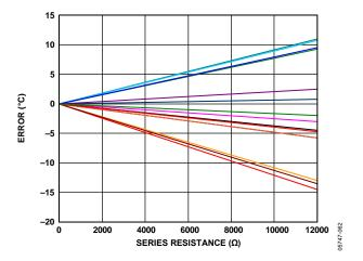
Figure 31. Temperature Error vs. Series Resistance for 15 Typical Devices
