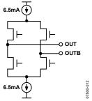
Figure 9. LVDS Output Simplified Equivalent Circuit
