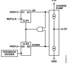
Figure 10. PFD Simplified Schematic and Timing (in Lock)
