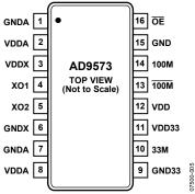
Figure 5. Pin Configuration
