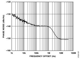
Figure 7. 33.33 MHz Phase Noise
