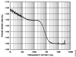
Figure 6. 100 MHz Phase Noise
