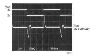
Figure 4. LT1790-2.5 Sourcing and Sinking 0.5mA
