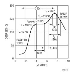
Figure 10. Lead-Free Reflow Profile
