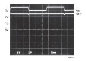
Figure 2. Output Response to 0.5V Ripple on VIN
