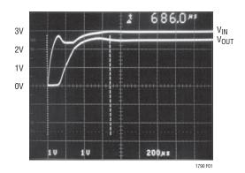
Figure 1. Turn-On Characteristics of LT1790-2.5
