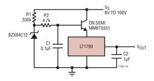
Figure 14. Extended Supply Range Reference
