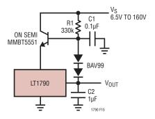
Figure 15. Extended Supply Range Reference
