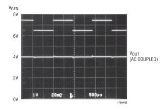
Figure 6. LT1790-2.5 Sinking -4mA to -5mA
