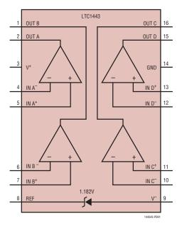
**OUT B (Pin 1):** Comparator B Output. (Open-drain output for LTC1444). Output can source up to 40mA (LTC1443, LTC1445) and sink 5mA.
