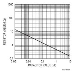
Figure 2. Damping Resistance vs Bypass Capacitor Value
