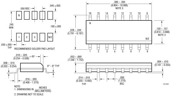
3. THESE DIMENSIONS DO NOT INCLUDE MOLD FLASH OR PROTRUSIONS. MOLD FLASH OR PROTRUSIONS SHALL NOT EXCEED .006" (0.15mm)
