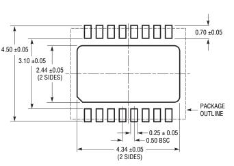
**DHD Package** 16-Lead Plastic DFN (5mm × 4mm) (Reference LTC DWG # 05-08-1707)
