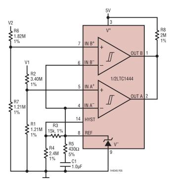
Figure 5. Glitch-Free Level Detector with Hysteresis
