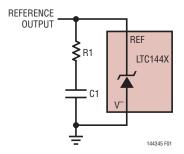
Figure 1. Damping the Reference Output
