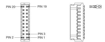
Order kit part number 73-788-002 for control connector interface with unloaded housing and 20 pins
