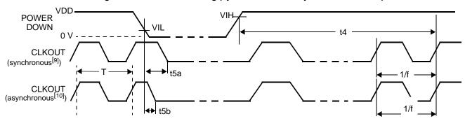
Figure 5. Power-up Timing
