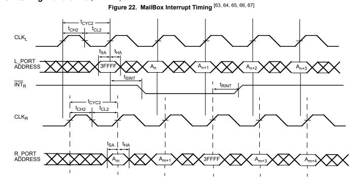
66. At least one byte enable  $(\overline{B0}-\overline{B3})$  is required to be active during interrupt operations.
