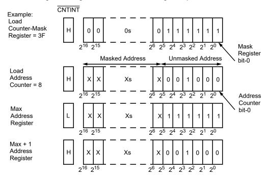
Figure 5. Programmable Counter-Mask Register Operation <sup>[19, 20]</sup>
