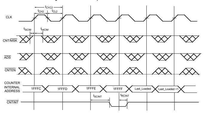
Figure 21. Counter Interrupt and Retransmit <sup>[58, 59, 60, 61, 62]</sup>
