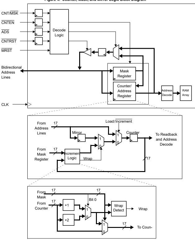
Figure 4. Counter, Mask, and Mirror Logic Block Diagram <sup>[18]</sup>
