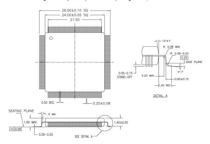
Figure 26. 176-pin TQFP (24 × 24 × 1.4 mm) Package Outline, 51-85132
