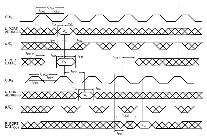
Figure 20. Left\_Port (L\_Port) Write to Right\_Port (R\_Port) Read <sup>[55, 56, 57]</sup>
