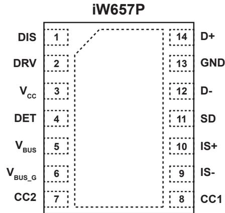
**Figure 4.1 : 14-Lead TDFN 4x3mm Package
