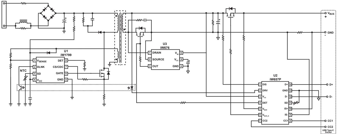
**Figure 3.3 : iW657P Typical Application Circuit with Secondary-Side Current Sensing
