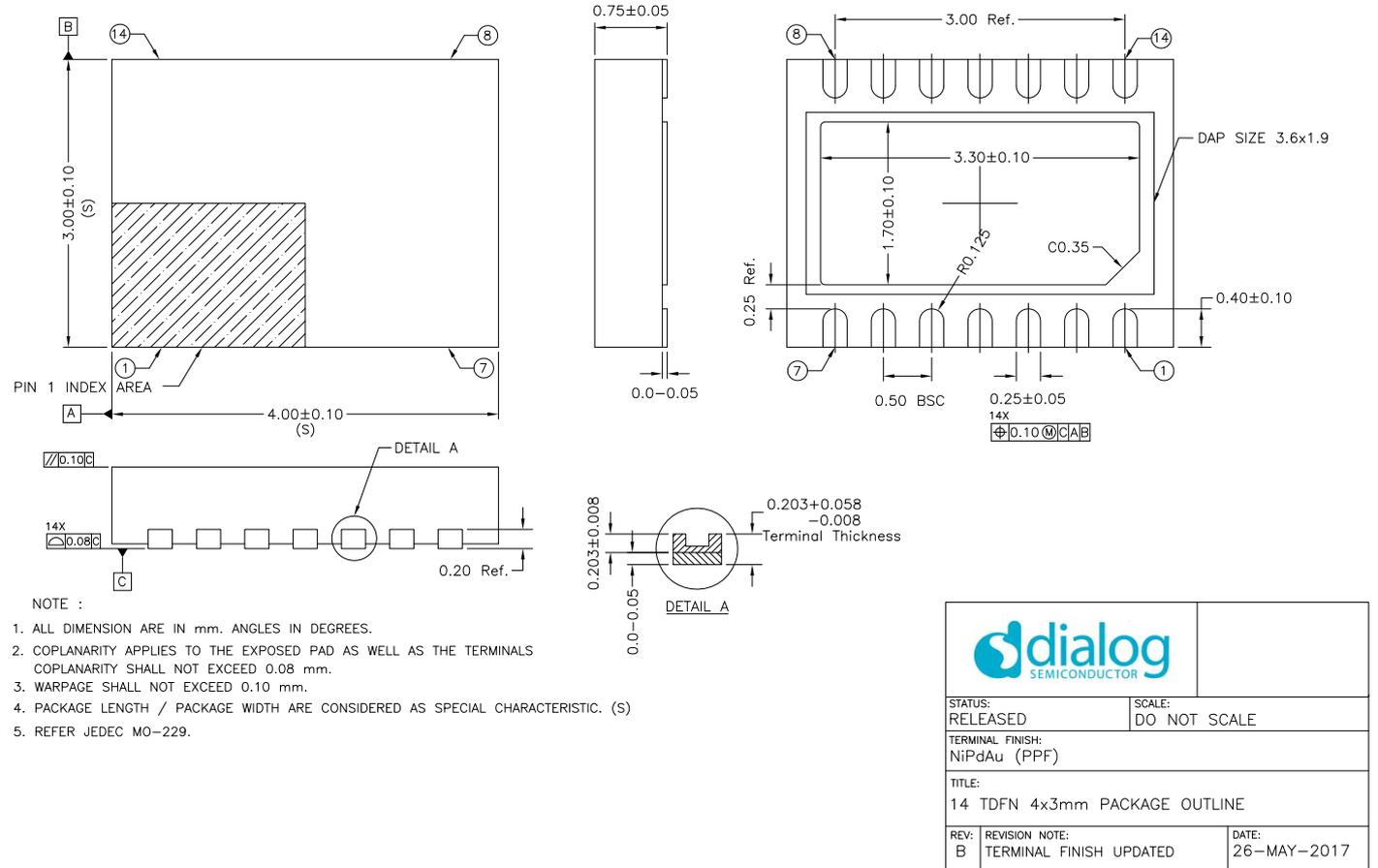
**Figure 6.1 : 14-Lead TDFN 4x3mm Package**
