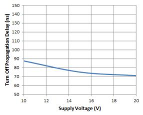
Figure 5. Turn-off Propagation Delay vs. Supply Voltage
