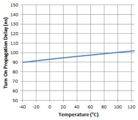
Figure 4. Turn-on Propagation Delay vs. Temperature
