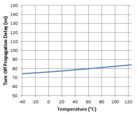
Figure 6. Turn-off Propagation Delay vs. Temperature
