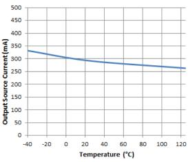
Figure 14. Output Source Current vs. Temperature
