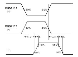
Figure 2. Switching Time Waveform Definitions
