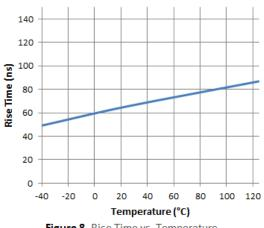
Figure 8. Rise Time vs. Temperature
