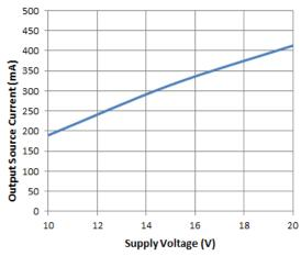
Figure 13. Output Source Current vs. Supply Voltage
