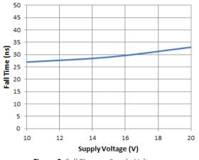
Figure 9. Fall Time vs. Supply Voltage
