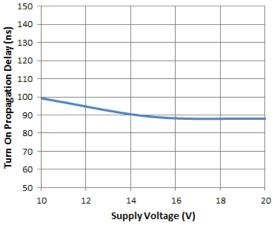
Figure 3. Turn-on Propagation Delay vs. Supply Voltage
