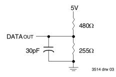
Figure 1. AC Test Load
