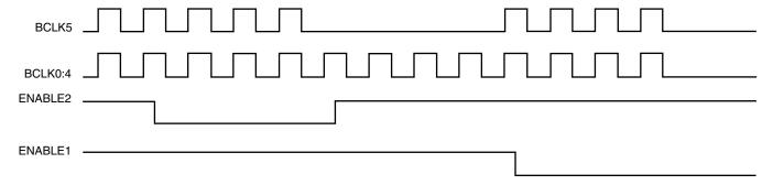
Figure 1. Enable Timing Diagram
