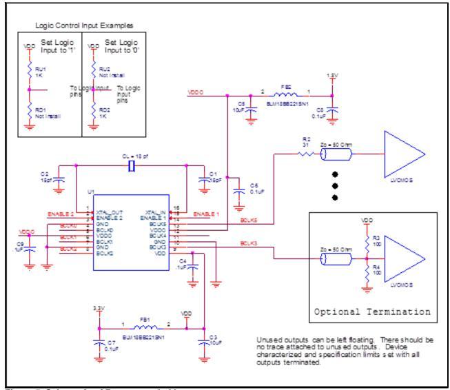
Figure 5. Schematic of Recommended Layout
