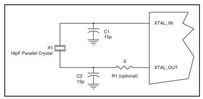
Figure 2. Crystal Input Interface
