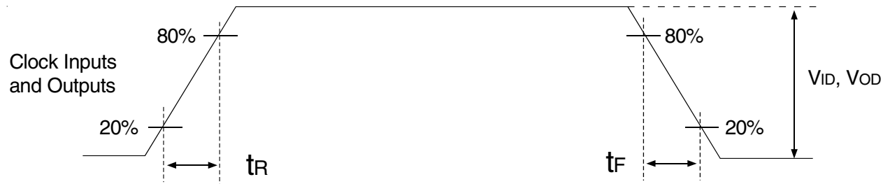
Figure 8. Input and Output Slew Rates
