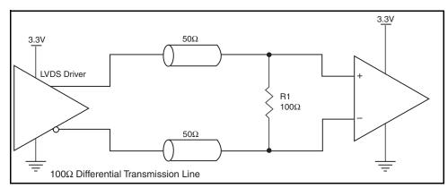
Figure 3. Typical LVDS Driver Termination
