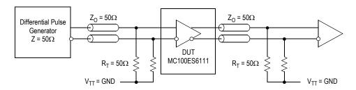
Figure 3. MC100ES6111 AC Test Reference
