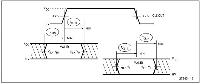
Figure 10. Input Setup and Hold
