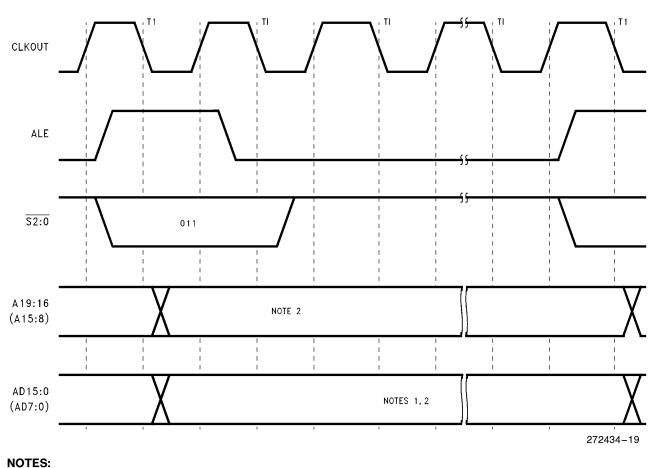
1. Address information is invalid. If previous bus cycle was a read, then the AD15:0 (AD7:0) lines will float during T1. Otherwise, the AD15:0 (AD7:0) lines will continue to drive during T1 (data is invalid). All other control lines are in their inactive state.
