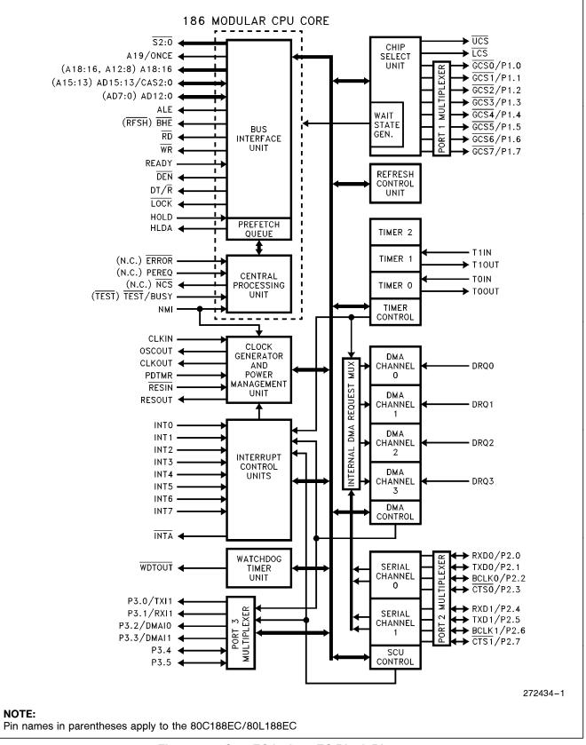
Figure 1. 80C186EC/80L186EC Block Diagram
