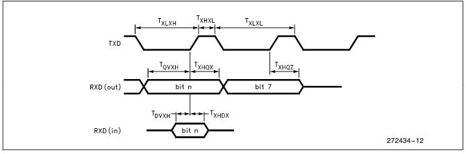
Figure 13. Serial Port Mode 0 Waveform
