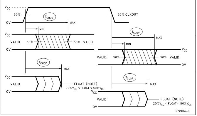
Figure 9. Output Delay and Float Waveforms
