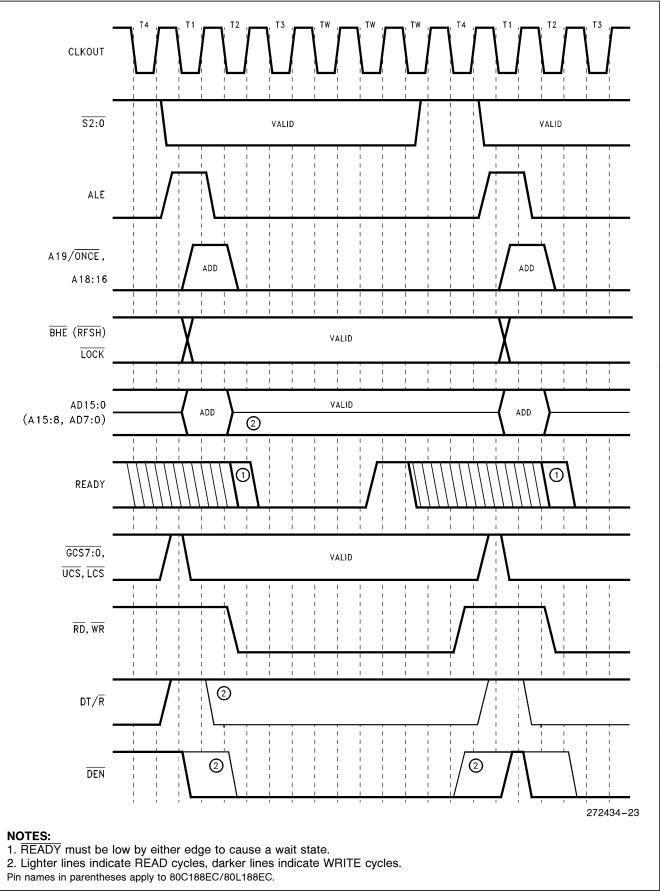
Figure 24. READY Cycle Waveforms
