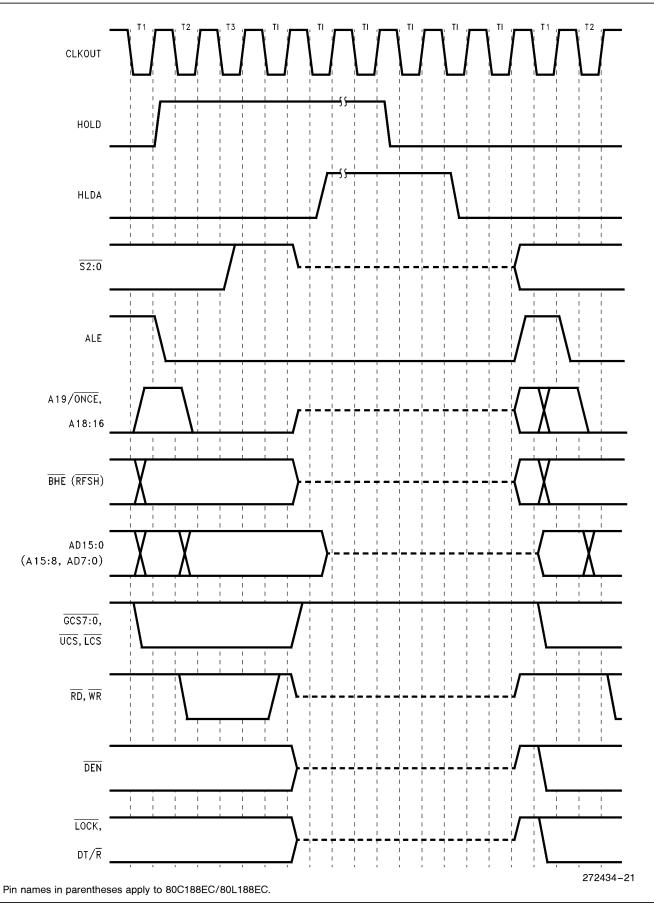
Figure 22. HOLD/HLDA Cycle Waveforms
