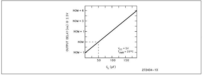
Figure 14. Typical Output Delay Variations versus Load Capacitance
