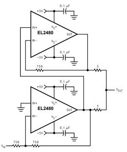
INVERTING 200mA OUTPUT CURRENT DISTRIBUTION AMPLIFIER
