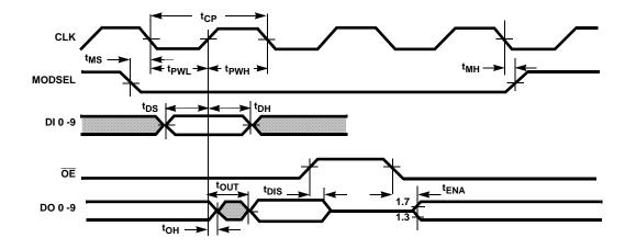
FIGURE 5. FUNCTIONAL TIMING (CLKSEL = HIGH)
