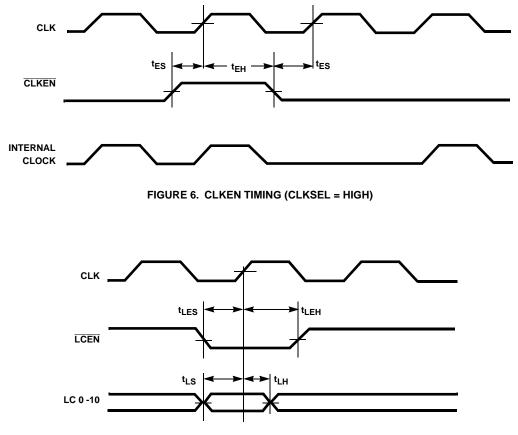
FIGURE 7. LENGTH CONTROL TIMING (CLKSEL = HIGH)
