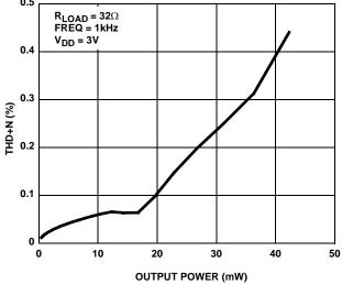
FIGURE 12. THD+N vs OUTPUT VOLTAGE
