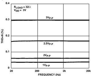
FIGURE 11. THD+N vs SIGNAL LEVELS vs FREQUENCY
