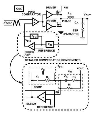
FIGURE 5. VOLTAGE-MODE BUCK CONVERTER COMPENSATION DESIGN
