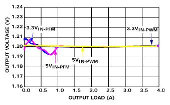
FIGURE 10. VOUT REGULATION vs LOAD (1MHz,  $V_{OUT} = 1.2V)$
