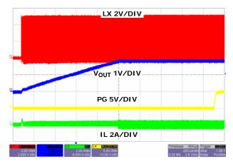
FIGURE 34. OUTPUT SHORT CIRCUIT RECOVERY
