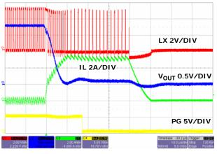
FIGURE 33. OUTPUT SHORT CIRCUIT
