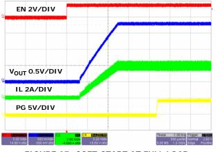
FIGURE 27. SOFT-START AT FULL LOAD
