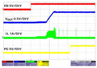
FIGURE 26. SOFT-START WITH PRE-BIASED 1V
