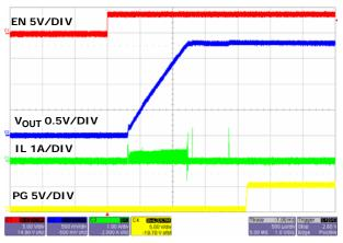
FIGURE 25. SOFT-START AT NO LOAD (PFM)
