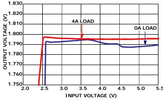
FIGURE 16. OUTPUT VOLTAGE REGULATION vs VIN (PFM  $V_{OUT} = 1.8V$ )
