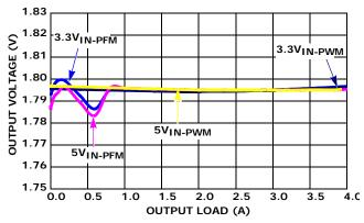
FIGURE 12. VOUT REGULATION vs LOAD (1MHz,  $V_{OUT} = 1.8V$
