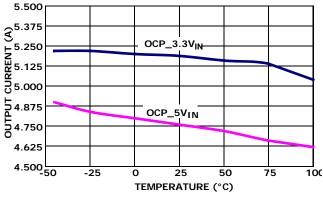
FIGURE 35. OUTPUT CURRENT LIMIT vs TEMPERATURE
