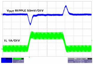
FIGURE 22. LOAD TRANSIENT (PWM)
