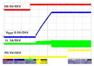
FIGURE 24. SOFT-START WITH NO LOAD (PWM)
