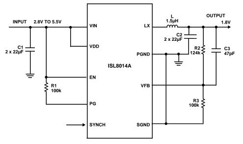
FIGURE 1. TYPICAL APPLICATION DIAGRAM
