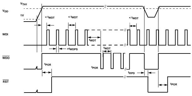
FIGURE 5. WATCHDOG TIMING DIAGRAM
