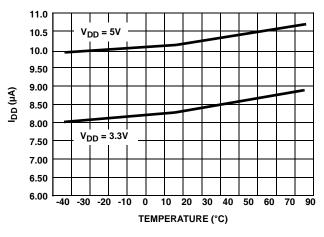
FIGURE 6. I<sub>DD</sub> vs TEMPERATURE
