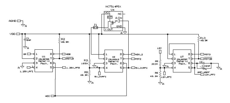
FIGURE 17. ISL88705EVAL1 SCHEMATIC (TOP BANK)
