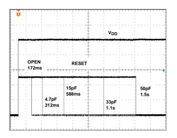
FIGURE 11. RESET ASSERTION vs CPOR
