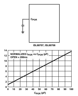
FIGURE 3. ADJUSTING tPOR WITH A CAPACITOR
