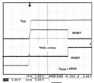
FIGURE 10. RESET AND RESET ASSERTION
