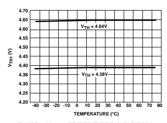
FIGURE 7. V<sub>TH1</sub> vs TEMPERATURE FOR 5V SUPPLY
