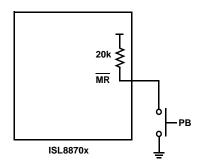
FIGURE 4. CONNECTING A MANUAL RESET PUSH-BUTTON
