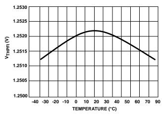
FIGURE 9. V<sub>THPFI</sub> vs TEMPERATURE
