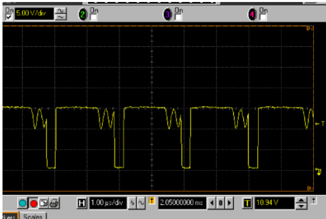
FIGURE 7. BOOST SWITCH NODE AT 100mA (PARTIAL DISCONTINUOUS)
