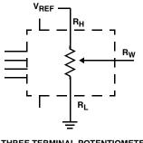
THREE TERMINAL POTENTIOMETER; VARIABLE VOLTAGE DIVIDER
