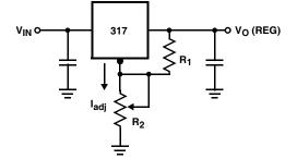
$V_{O}$  (REG) = 1.25V (1+R<sub>2</sub>/R<sub>1</sub>)+I<sub>adj</sub> R<sub>2</sub>
