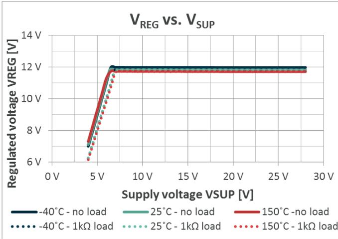
Figure 10-7 MLX83202 Regulated output voltage vs. supply voltage
