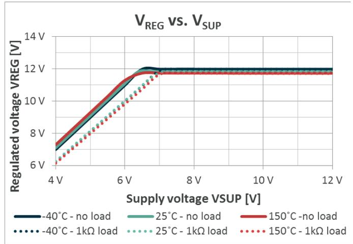
Figure 10-8 MLX83202 Regulated output voltage vs. supply voltage
