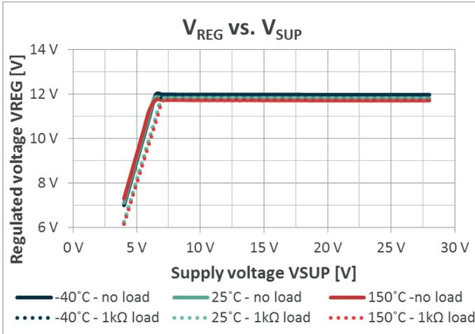
Figure 10-1 MLX83203 Regulated output voltage vs. supply voltage
