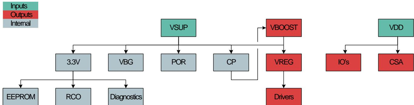
Figure 12-1 Principle organization of the supply system
