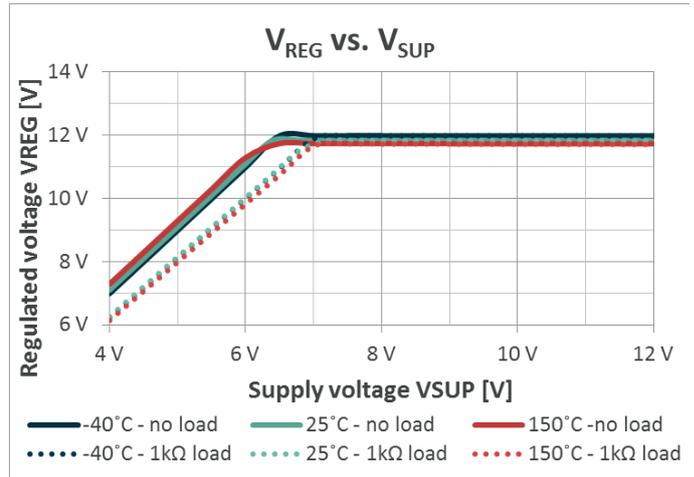
Figure 10-2 MLX83203 Regulated output voltage vs. supply voltage
