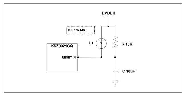
The following reset circuit is recommended for applications where reset is driven by another device (e.g., CPU or FPGA). At power-on-reset, R, C and D1 provide the necessary ramp rise time to reset the KSZ9021GQ device. The RST\_OUT\_N from CPU/FPGA provides the warm reset after power up.
