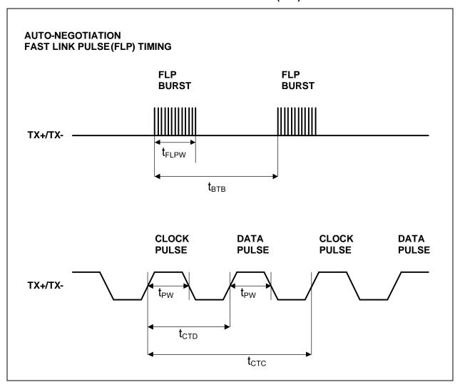
TABLE 6-5: AUTO-NEGOTIATION FAST LINK PULSE (FLP) TIMING PARAMETERS
