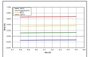
FIGURE 38-97: FVR Voltage Error 4x, PIC16F15324/44 Only.
