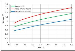
FIGURE 38-100: Input Level TTL.
