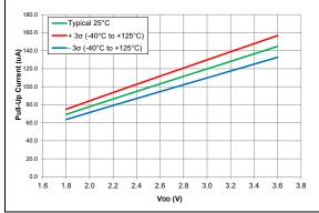
FIGURE 38-31: Weak Pull-up Current, PIC16LF15324/44 Only.
