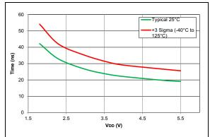
FIGURE 38-102: Fall Time, Slew Rate Control Enabled.
