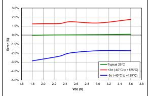
FIGURE 38-27: HFINTOSC Typical, Frequency Error, PIC16LF15324/44 Only.
