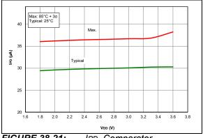
FIGURE 38-21: IPD, Comparator, PIC16LF15324/44 Only.
