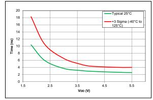
*FIGURE 38-104:* Fall Time, Slew Rate Control Disabled.
