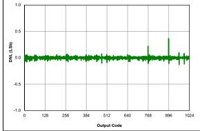
**FIGURE 38-49:** ADC 10-bit Mode, Single-Ended DNL, VDD = 3.0V, VREF = 3.0V, TAD = 4  $\mu$ S, 25°C.
