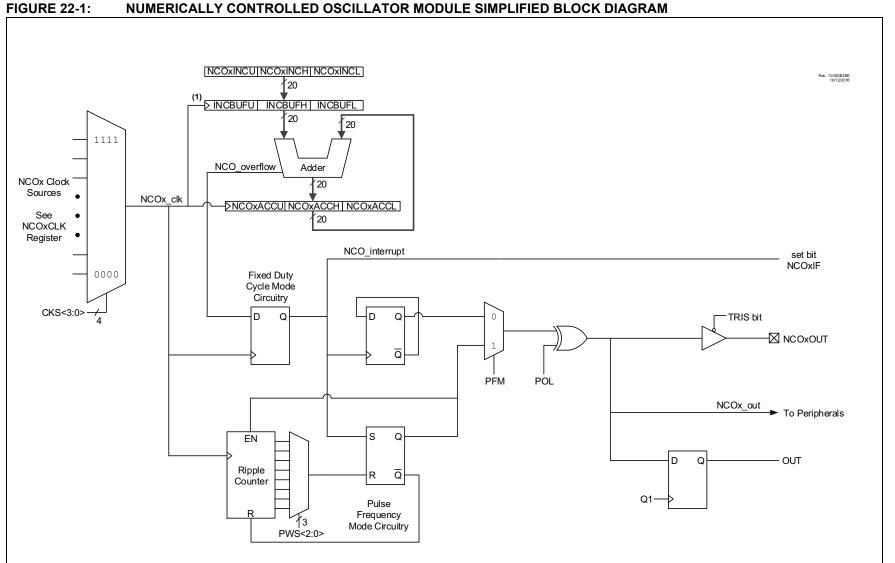
Note 1: The increment registers are double-buffered to allow for value changes to be made without first disabling the NCO module. The full increment value is loaded into the buffer registers on the second rising edge of the NCOx clk signal that occurs immediately after a write to NCOxINCL register. The buffers are not user-accessible and are shown here for reference.
