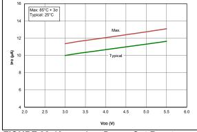
FIGURE 38-19: IPD, Brown-Out Reset (BOR), BORV = 1, PIC16F15324/44 Only.
