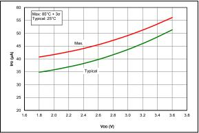
**FIGURE 38-16:** IPD, Fixed Voltage Reference (FVR), PIC16LF15324/44 Only.
