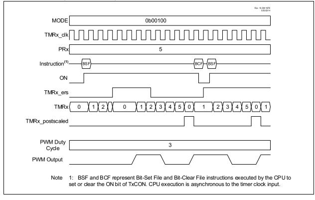
When the timer is used in conjunction with the CCP in PWM mode then an early Reset shortens the period and restarts the PWM pulse after a two clock delay. Refer to Figure 27-6.
