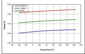
**FIGURE 38-40:** Brown-Out Reset Voltage, Trip Point (BORV = 1), PIC16LF15324/44 Only.
