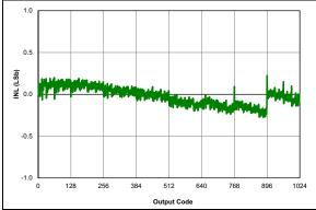
**FIGURE 38-51:** ADC 10-bit Mode, Single-Ended INL, VDD = 3.0V, VREF = 3.0V, TAD = 1  $\mu$ S, 25°C.
