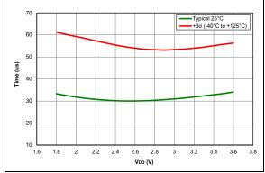
FIGURE 38-91: Band Gap Ready Time, PIC16LF15324/44 Only.
