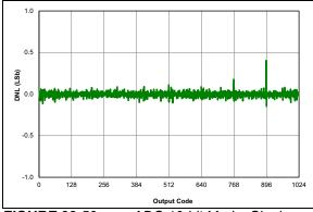
**FIGURE 38-50:** ADC 10-bit Mode, Single-Ended DNL, VDD = 3.0V, VREF = 3.0V,  $TAD = 8 \mu S$ , 25°C.
