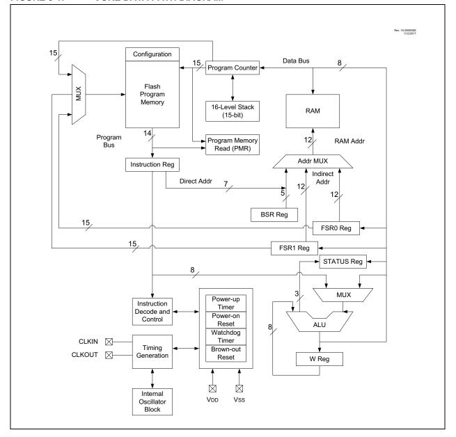
The hardware stack is 16-levels deep and has Overflow and Underflow Reset capability. Direct, Indirect, and Relative Addressing modes are available. Two File Select Registers (FSRs) provide the ability to read program and data memory.
