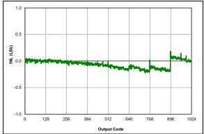
**FIGURE 38-52:** ADC 10-bit Mode, Single-Ended INL, VDD = 3.0V, VREF = 3.0V, TAD = 4  $\mu$ S, 25°C.
