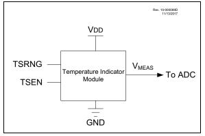
The output of the circuit is measured using the internal Analog-to-Digital Converter. A channel is reserved for the temperature circuit output. Refer to Section 20.0 "Analog-to-Digital Converter (ADC) Module" for detailed information.
