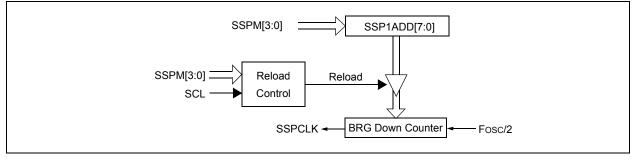
**Note:** Values of 0x00, 0x01 and 0x02 are not valid for SSP1ADD when used as a Baud Rate Generator for I<sup>2</sup>C. This is an implementation limitation.
