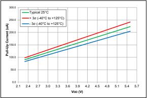
FIGURE 38-30: Weak Pull-up Current, PIC16F15324/44 Only.
