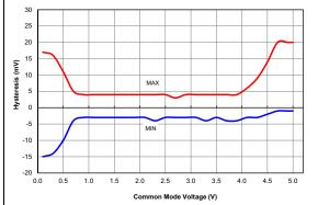
**FIGURE 38-81:** Comparator Offset, NP Mode (CxSP = 1), VDD = 5.5V, Typical Measured Values at 25°C.
