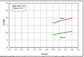
**FIGURE 38-18:** IPD, Brown-Out Reset (BOR), BORV = 1, PIC16LF15324/44 Only.
