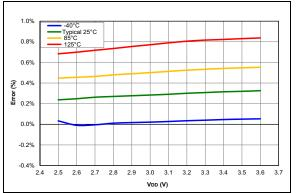
FIGURE 38-95: FVR Voltage Error 2x, PIC16LF15324/44 Only.
