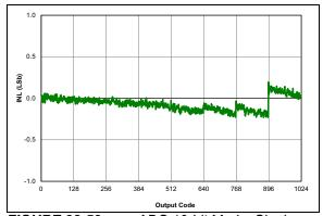
**FIGURE 38-53:** ADC 10-bit Mode, Single-Ended INL, VDD = 3.0V, VREF = 3.0V, TAD = 8  $\mu$ S, 25°C.
