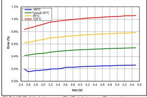
FIGURE 38-94: FVR Voltage Error 1x, PIC16F15324/44 Only.
