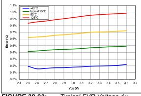
FIGURE 38-93: Typical FVR Voltage 1x, PIC16LF15324/44 Only.
