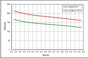
**FIGURE 38-86:** Comparator Response Time Falling Edge, PIC16F15324/44 Only.
