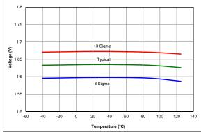
FIGURE 38-107: POR Rearm Voltage, NP Mode, PIC16F15324/44 Only.
