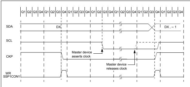
FIGURE 32-23: CLOCK SYNCHRONIZATION TIMING
