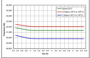
FIGURE 38-26: LFINTOSC Frequency, PIC16F15324/44 Only.
