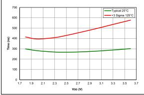
**FIGURE 38-87:** Comparator Response Time Rising Edge, PIC16LF15324/44 Only.
