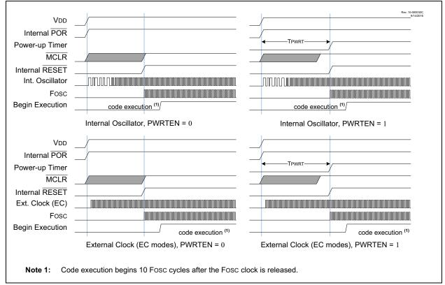
FIGURE 8-3: RESET START-UP SEQUENCE
