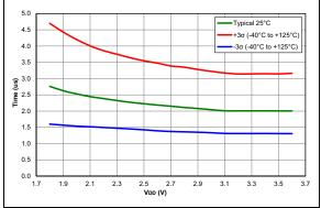
FIGURE 38-66: ADC RC Oscillator Period, PIC16LF15324/44 Only.
