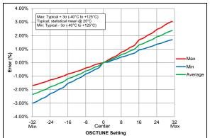
FIGURE 38-105: OSCTUNE Center Frequency, PIC16LF15324/44 Only.
