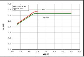
FIGURE 38-6: IDD, HFINTOSC Mode, Fosc = 32 MHz, PIC16F15324/44 Only.
