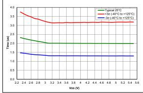
FIGURE 38-67: ADC RC Oscillator Period, PIC16F15324/44 Only.
