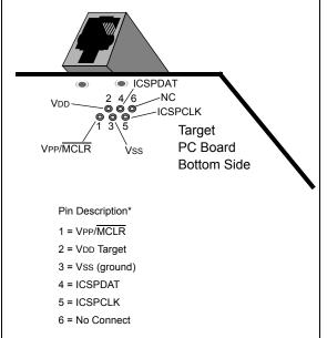
Another connector often found in use with the PICkit<sup>™</sup> programmers is a standard 6-pin header with 0.1 inch spacing. Refer to Figure 35-2.
