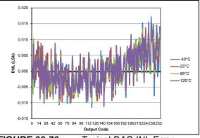
**FIGURE 38-70:** Typical DAC INL Error, VDD = 5.0V, VREF = External 3V.
