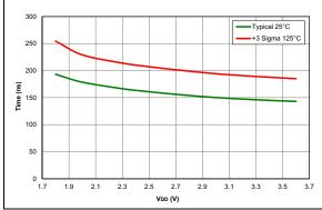
FIGURE 38-85: Comparator Response Time Falling Edge, PIC16LF15324/44 Only.
