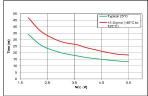
FIGURE 38-101: Rise Time, Slew Rate Control Enabled.
