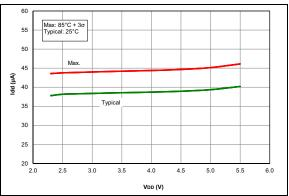
FIGURE 38-17: IPD, Fixed Voltage Reference (FVR), PIC16F15324/44 Only.
