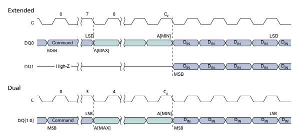
Notes: 1. For extended-SPI protocol,  $C_x = 7 + (A[MAX] + 1)$ ; For dual-SPI protocol,  $C_x = 3 + (A[MAX] + 1)/2$ .
