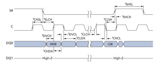
Figure 56: Write Protect Setup and Hold During WRITE STATUS REGISTER Operation (SRWD = 1)
