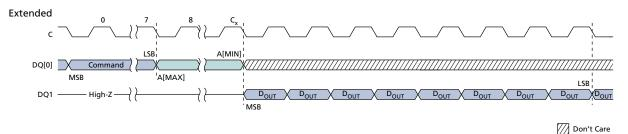
Notes: 1. For extended protocol,  $C_x = 7 + (A[MAX] + 1)$ ; For dual protocol,  $C_x = 3 + (A[MAX] + 1)/2$ ; For quad protocol,  $C_x = 1 + (A[MAX] + 1)/4$ .
