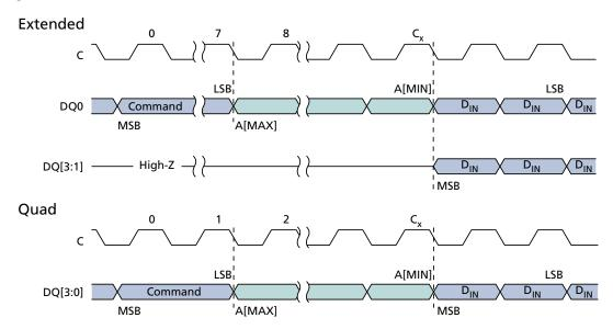
Notes: 1. For extended-SPI protocol,  $C_x = 7 + (A[MAX] + 1)$ ; For quad-SPI protocol,  $C_x = 1 + (A[MAX] + 1)/4$ .
