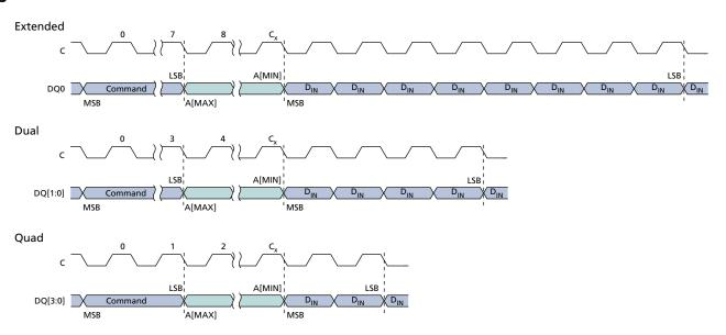
Notes: 1. For extended-SPI protocol,  $C_x = 7 + (A[MAX] + 1)$ ; For dual-SPI protocol,  $C_x = 3 + (A[MAX] + 1)/2$ ; For quad-SPI protocol,  $C_x = 1 + (A[MAX] + 1)/4$ .
