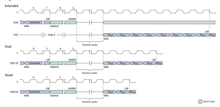
Notes: 1. For extended protocol,  $C_x = 7 + (A[MAX] + 1)$ ; For dual protocol,  $C_x = 3 + (A[MAX] + 1)/2$ ; For quad protocol,  $C_x = 1 + (A[MAX] + 1)/4$ .
