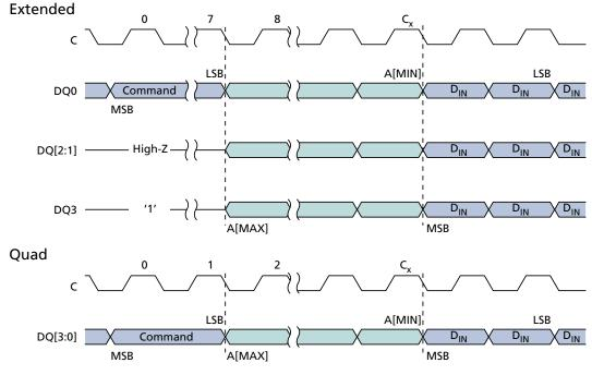
lotes: 1. For extended-SPI protocol,  $C_x = 7 + (A[MAX] + 1)/4$ ; For quad-SPI protocol,  $C_x = 1 + (A[MAX] + 1)/4$ .
