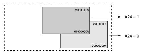
The PROGRAM and ERASE operations act upon the 128Mb segment selected in the extended address register. The BULK ERASE operation erases the entire device.
