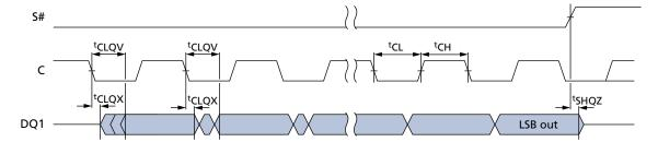
**Figure 59: Output Timing for DTR**
