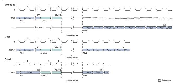
Note: 1. For extended-SPI protocol,  $C_x = 7 + (A[MAX] + 1)$ ; For dual-SPI protocol,  $C_x = 3 + (A[MAX] + 1)/2$ ; For quad-SPI protocol,  $C_x = 1 + (A[MAX] + 1)/4$ .
