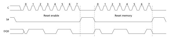
Figure 54: Serial Input Timing STR
