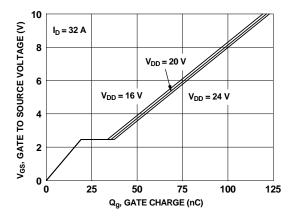
Figure 7. Gate Charge Characteristics
