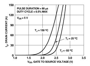
Figure 5. Transfer Characteristics
