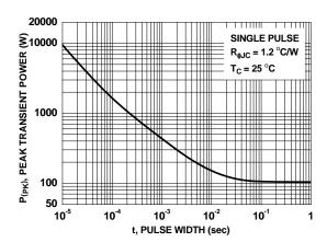
Figure 12. Single Pulse Maximum Power Dissipation
