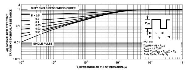
Figure 13. Transient Thermal Response Curve
