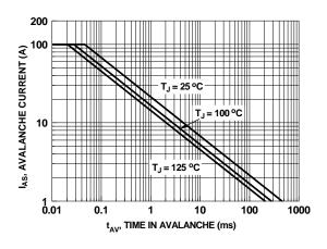
Figure 9. Unclamped Inductive Switching Capability
