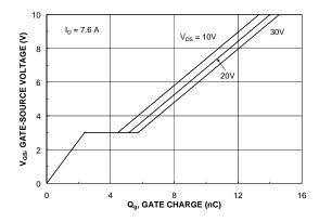
Figure 7. Gate Charge Characteristics.
