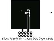
50°C/W when mounted on a 1in<sup>2</sup> pad of 2 oz copper
