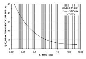
Figure 11. Single Pulse Maximum Peak Current.
