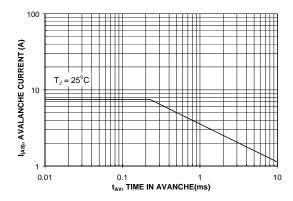
Figure 12. Unclamped Inductive Switching Capability.
