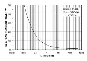
Figure 10. Single Pulse Maximum Power Dissipation.
