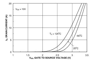
Figure 5. Transfer Characteristics.
