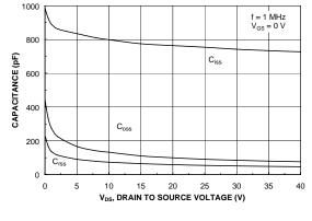
Figure 8. Capacitance Characteristics.
