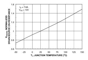
Figure 3. On-Resistance Variation with Temperature.
