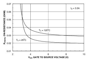
Figure 4. On-Resistance Variation with Gate-to-Source Voltage.
