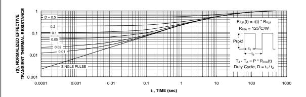
Figure 25. Transient Thermal Response Curve.
