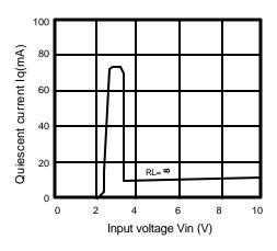
Figure 2.Quiescent Current vs. Input Voltage
