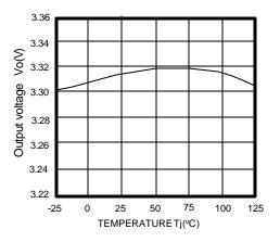
Figure 4.Output Voltage vs. Temperature(Tj)
