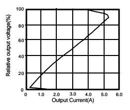
Figure 8. Overcurrent Protection Characteristics (Typical Value)
