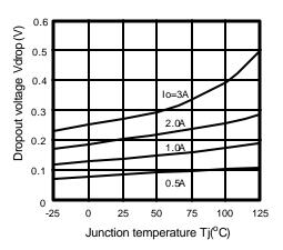
Figure 6.Dropout Voltage vs. Junction Temperature
