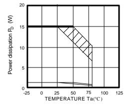
Figure 7.Power Dissipation vs. Temperature(Ta)
