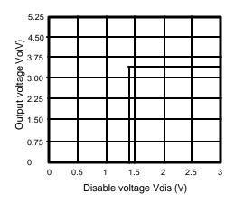
Figure 3.Output Voltage vs. Disable Voltage
