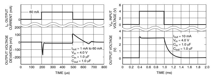
Figure 10. Load Transient Response
