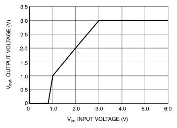
Figure 12. Output Voltage vs. Input Voltage
