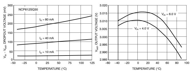
Figure 2. Dropout Voltage vs. Temperature
