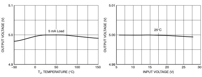
Figure 5. Output Voltage vs. Temperature
