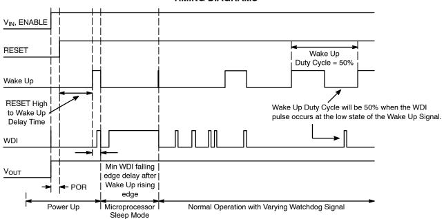
Figure 2. Power Up, Sleep Mode and Normal Operation
