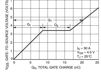
Figure 8. Gate-To-Source and Drain-To-Source Voltage vs. Total Charge
