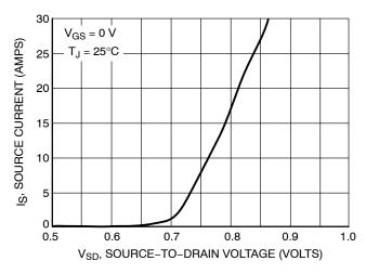
Figure 10. Diode Forward Voltage vs. Current
