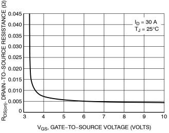
Figure 3. On–Resistance vs. Gate–to–Source Voltage
