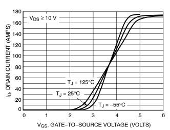
Figure 2. Transfer Characteristics
