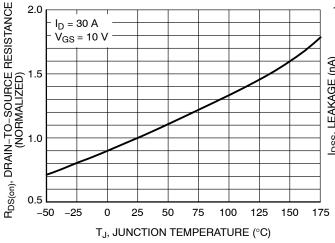
Figure 5. On–Resistance Variation with Temperature
