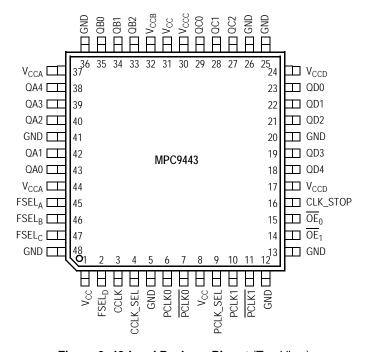
Figure 2. 48-Lead Package Pinout (Top View)
