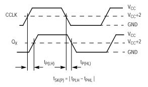
Figure 15. Output Pulse Skew (t<sub>SK(P)</sub>) Test Reference
