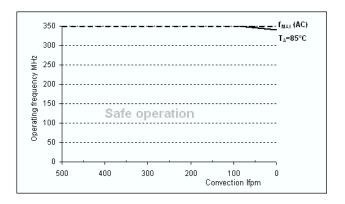
Figure 8. Maximum MPC9443 Frequency, V<sub>CC</sub> = 3.3 V, MTBF 4 Years, Driving Series Terminated Transmission Lines
