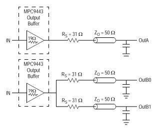
Figure 3. Single versus Dual Transmission Lines
