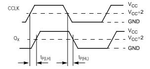
Figure 13. Propagation Delay (t<sub>PD</sub>) Test Reference
