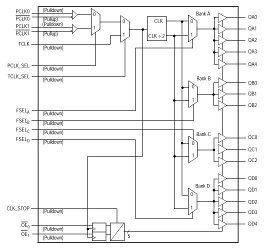
Figure 1. MPC9443 Logic Diagram
