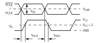
Figure 12. Propagation Delay (t<sub>PD</sub>) Test Reference
