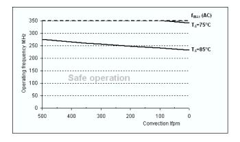
Figure 6. Maximum MPC9443 frequency, V<sub>CC</sub> = 3.3 V, MTBF 9.1 Years, Driving Series Terminated Transmission Lines
