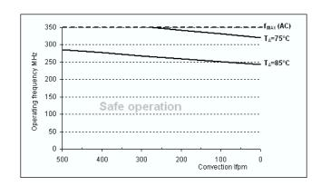
Figure 9. Maximum MPC9443 Frequency, V<sub>CC</sub> = 3.3 V, MTBF 4 Years, 4 pF Load per Line
