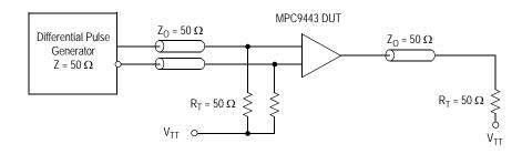
Figure 11. PCLK MPC9443 AC Test Reference
