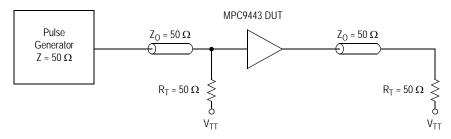
Figure 10. CCLK MPC9443 AC Test Reference for  $V_{cc}$  = 3.3 V and  $V_{cc}$  = 2.5 V
