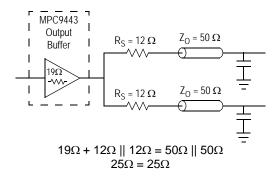
Figure 5. Optimized Dual Line Termination
