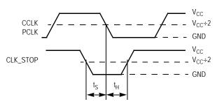
Figure 19. Setup and Hold Time ( $t_S$ ,  $t_H$ ) Test Reference
