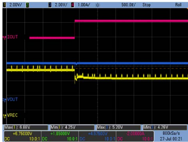
Figure 11. Load Transient: V OUT = 5V, 0A → 1.2A
