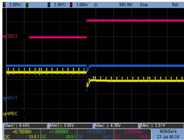
Figure 13. Load Transient: V_{OUT} = 4.5V, 0A \rightarrow 1.2A
