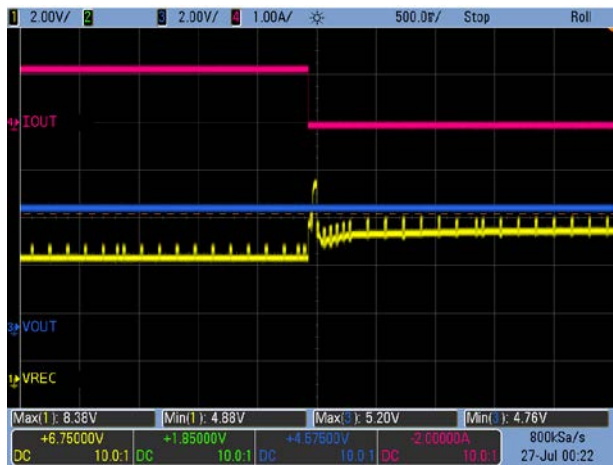
Figure 12. Load Transient: V OUT = 5V, 1.2A → 0A
