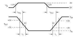
Figure 4. Driver Propagation Delay and Transition Time Waveforms Slew Rate (SR) =  $6V/(t_r \text{ or } t_f)$
