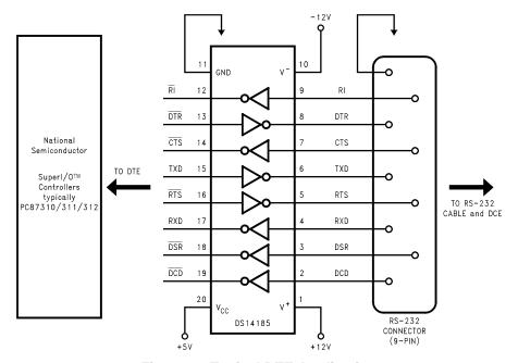
Figure 7. Typical DTE Application
