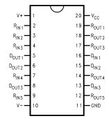
Figure 1. SOIC See Package DW0020B
