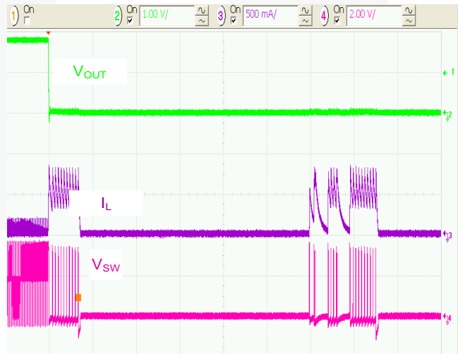
Figure 16. Metallic Short Applied at V OUT , 50μs/div.
