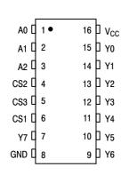
Figure 1. Pin Assignment
