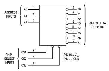
Figure 2. Logic Diagram
