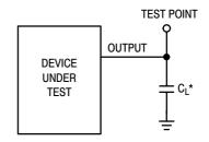
\*Includes all probe and jig capacitance
