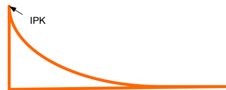
Figure 26. Input Charge Inrush Current
