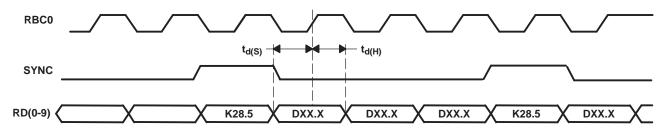
Figure 3. Synchronous Timing Characteristics Waveforms (TBI full-rate mode)
