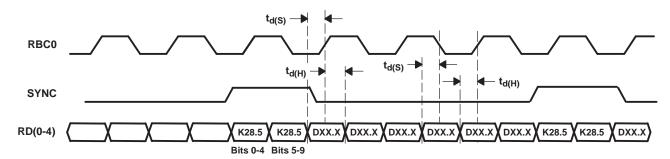
Figure 4. Synchronous Timing Characteristics Waveforms (DDR mode)
