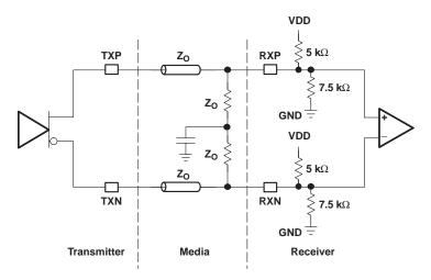
Figure 10. High-Speed I/O Directly-Coupled Mode
