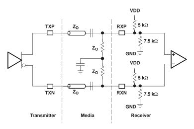
Figure 11. High-Speed I/O AC-Coupled Mode
