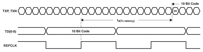
Figure 1. Transmitter Latency Full Rate Mode
