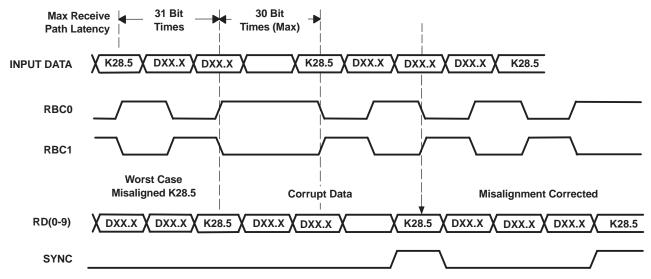
Figure 5. Word Realignment Timing Characteristics Waveforms
