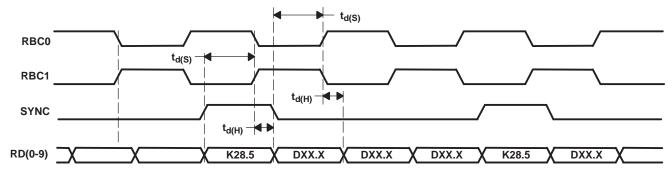
Figure 2. Synchronous Timing Characteristics Waveforms (TBI half-rate mode)
