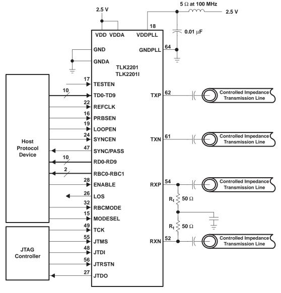
Figure 12. Typical Application Circuit (AC mode)
