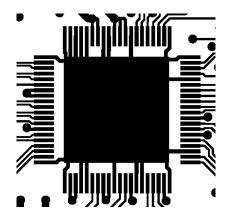
Figure 13. Example of a Thermal Land
