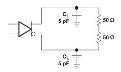
Figure 8. Transmitter Test Setup
