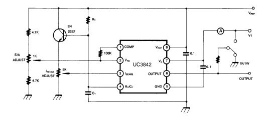
Figure 1. Open Loop Test Circuit
