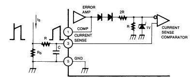
Figure 4. Current Sense Circuit
