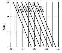
Figure 7. Timing Resistance vs Frequency
