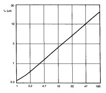
Figure 6. Oscillator Dead Time & Frequency
