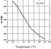
Figure 11. Temperature Drift (Ist)
