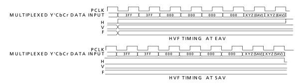
Figure 4-6: H:V:F Input Timing - HD 10-bit Input Mode
