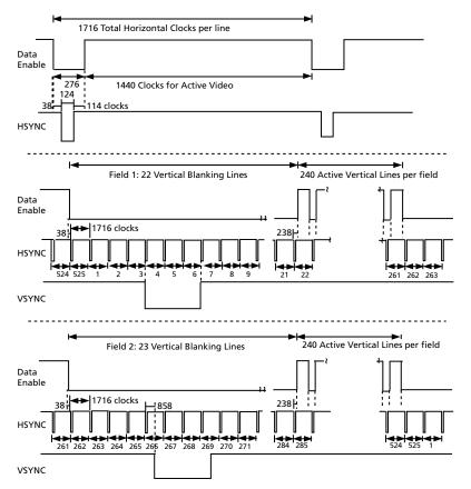
Figure 4-11: H:V:DE Input Timing 720 (1440) x 480i @ 59.94/60 (Format 6&7)
