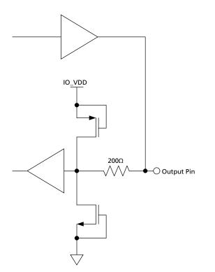
Figure 3-6: Bidirectional Digital Input/Output Pin with programmable drive strength. These pins are configured to input at all times except in test mode. (DIN0, DIN2, DIN3, DIN4, DIN5, DIN6, DIN7, DIN8, DIN9, DIN10, DIN11, DIN12, DIN13, DIN14, DIN15, DIN16, DIN17, DIN18, DIN19, DIN1)
