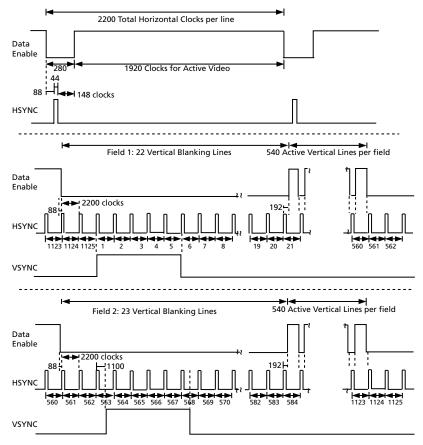
Figure 4-10: H:V:DE Input Timing 1920 x 1080i @ 59.94/60 (Format 5)
