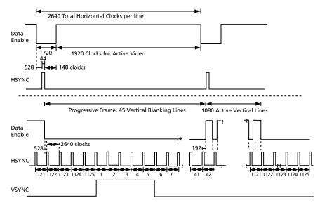
Figure 4-18: H:V:DE Input Timing 1920 x 1080p @ 25 (Format 33)
