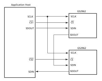
Figure 4-21: GSPI Application Interface Connection
