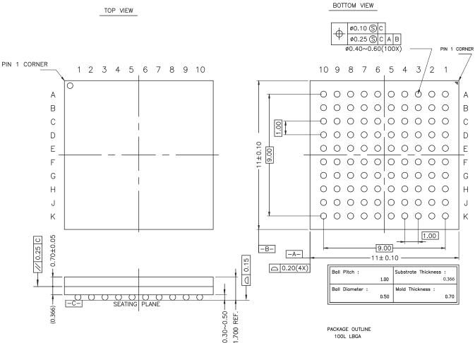
\* THE BALL DIAMETER, BALL PITCH, STAND-OFF & PACKAGE THICKNESS ARE DIFFERENT FROM JEDEC SPEC M0192 (LOW PROFILE BGA FAMILY) PACKAGE SIZE: 11 \* 11 \* 1.71 MM
