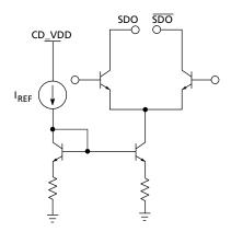
Figure 3-1: Differential Output Stage (SDO/SDO)
