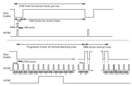
Figure 4-17: H:V:DE Input Timing 1920 x 1080p @ 23.94/24 (Format 32)
