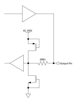
Figure 3-7: Bidirectional Digital Input/Output Pin with programmable drive strength. These pins are configured to output at all times except in reset mode. (LOCKED, SDOUT\_TDO, TDO)
