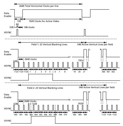
Figure 4-13: H:V:DE Input Timing 1920 x 1080i @ 50 (Format 20)
