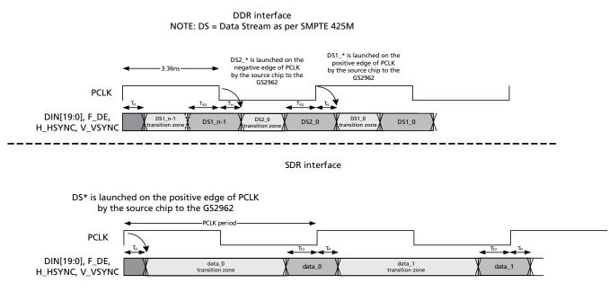
Figure 4-1: GS2962 Video Host Interface Timing Diagrams
