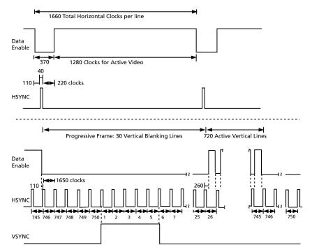
Figure 4-9: H:V:DE Input Timing 1280 x 720p @ 59.94/60 (Format 4)
