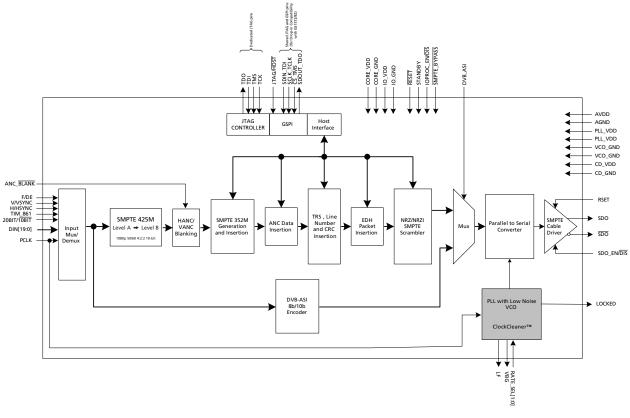
Figure A: GS2962 Functional Block Diagram
