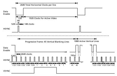
Figure 4-16: H:V:DE Input Timing 1920 x 1080p @ 50 (Format 31)
