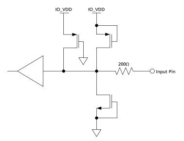
Figure 3-5: Digital Input Pin with weak pull-up - maximum pull-up current <110mA (CS\_TMS, SDO\_EN/DIS, TMS)
