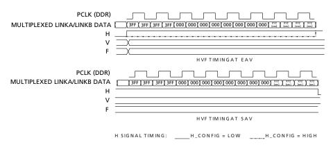
Figure 4-4: H:V:F Output Timing - 3G Level B 10-bit Mode
