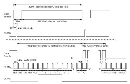
Figure 4-19: H:V:DE Input Timing 1920 x 1080p @ 29.97/30 (Format 34)
