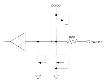
Figure 3-4: Digital Input Pin with weak pull-down - maximum pull-down current <110mA (JTAG/HOST, STANDBY, SCLK\_TCK, SDIN\_TDI, TCK, TDI)
