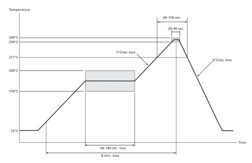
Figure 7-1: Pb-free Solder Reflow Profile
